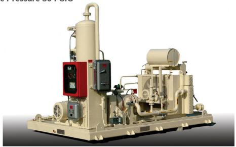
The TESCORP "CVR-1" SERIES is a completely self-contained compression system for applications for stock tank vapor recovery, flare gas recovery, or medium pressure process gas application. Constructed with a rugged rotary vane compressor and TESCORP vapor recovery technology and components, the CVR-1 is a complete and fully-automated system for applications that includes gas cooling, proportional capacity control, and sophisticated PLC driven control logic and communications.
