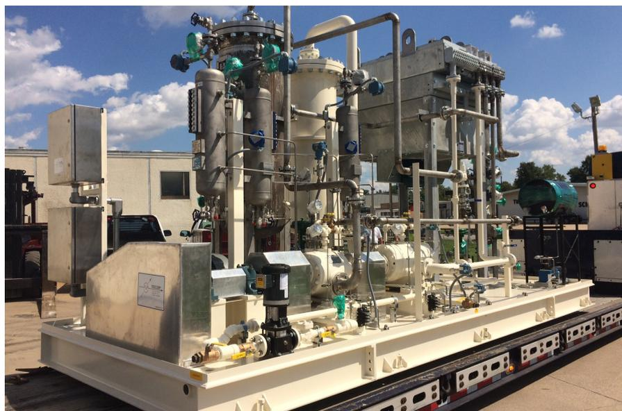
The TESCOP "CVR-2" SERIES is a completely self-contained two-stage compression system for applications for stock tank vapor recovery, flare gas recovery, or medium-pressure process gas application. Constructed with a rugged rotary vane compressor and TESCOP vapor recovery technology and components, the CVR-2 is a complete and fully-automated system for applications that require gas cooling, proportional capacity control, and sophisticated PLC driven control logic and communications.
