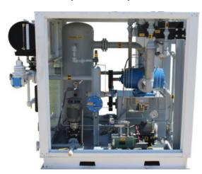
TESCORP "CVR-Modular" Series VRU system for application to meet EPA CFR 40, Subpart 0000 regulations and our customers stock tank vapor recovery gas emission requirements. Designed and constructed for "wet" gas applications utilizing a rugged single-stage rotary vane compressor. TESCORP's "CVR-M" & "CVR-MH" are compact, self-contained, fully-automated VRU systems complete with gas cooling, "load/no-load" capacity control with sophisticated PLC control logic with customer "DCS" communications.
