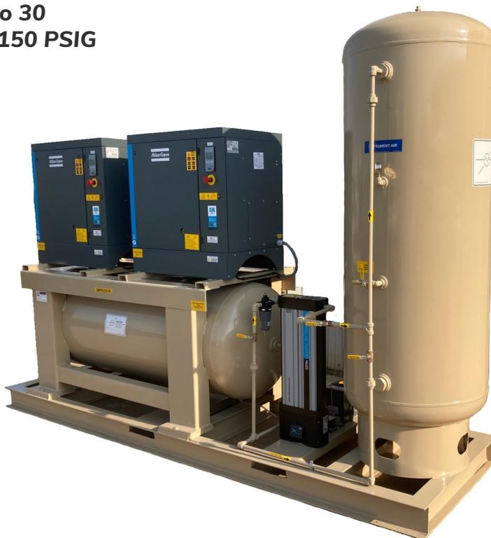
TESCORP “TIA-G” Series systems are designed and constructed for application to meet the rugged and harsh oilfield requirements for a continuous “instrument quality” air supply with 100% redundancy for critical operation. Designed and constructed with the Atlas Copco “G Series” Oil Flooded Rotary Screw compressor in a duplex 100% redundant configuration, the TESCORP TIA-G series provide continuous air supply with the capabilities to supply 200% flow rates upon demand.
