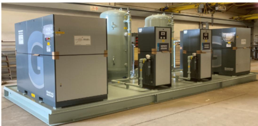
TESCORP "TIA-GA" Series systems are designed and constructed for application to meet the rugged and harsh oilfield requirements for a continuous "instrument quality" air supply with 100% redundancy for critical operation. Designed and constructed with the Atlas Copco "GA Series" Oil Flooded Rotary Screw compressor in a duplex 100% redundant configuration, the TESCOCORP TIA-G series provide continuous air supply with the capabilities to supply 200% flow rates upon demand.
